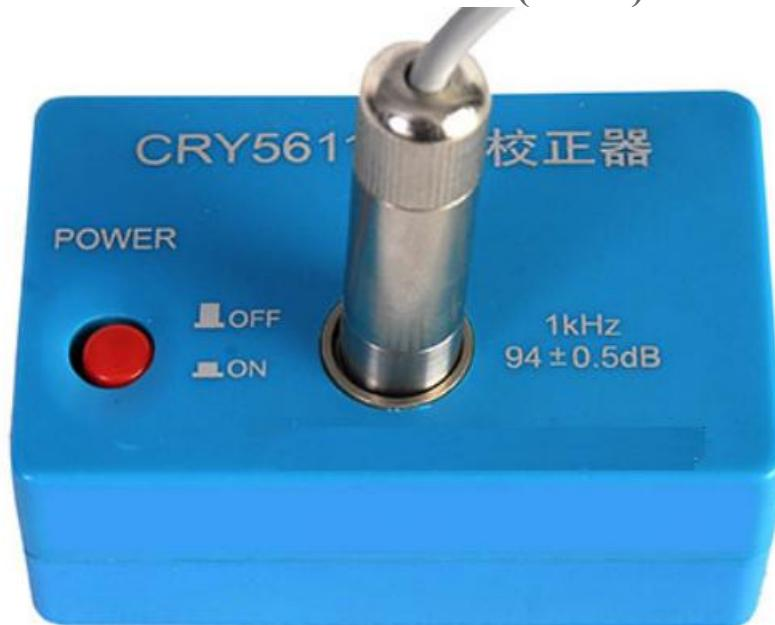
Suitable for calibrating sound pressure of sound level meter and electroacoustic measuring instrument. It has stable performance, compact size, light weight, energy saving and easy to use. Can produce 94dB standard sound pressure, frequency is 1000Hz. In accordance with IEC 60942:2003-2 and GB/T 15173:2010-2 standards. Calibration has nothing to do with the weight network used (A, B, C, D weight network attenuation is 0 at 1000Hz).
