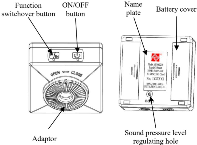
Figure 1 Calibrator Structural Diagram
