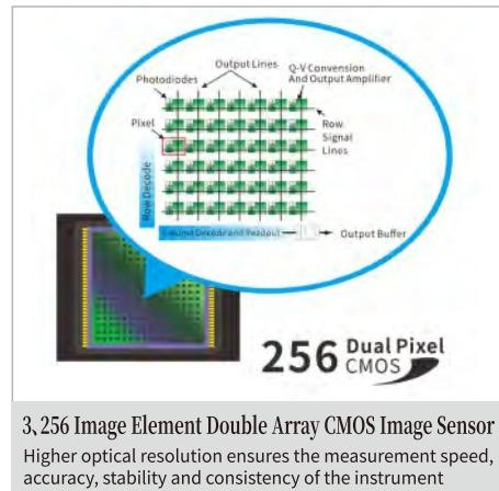
3. 256 Image Element Double Array CMOS Image Sensor
